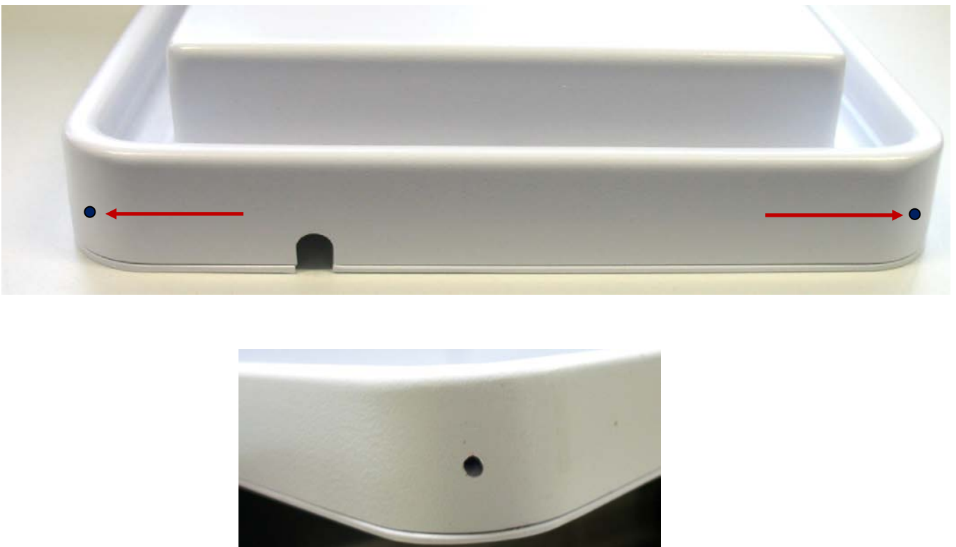
Figure 3: Draining holes at the bottom left- and right corner of the antenna
